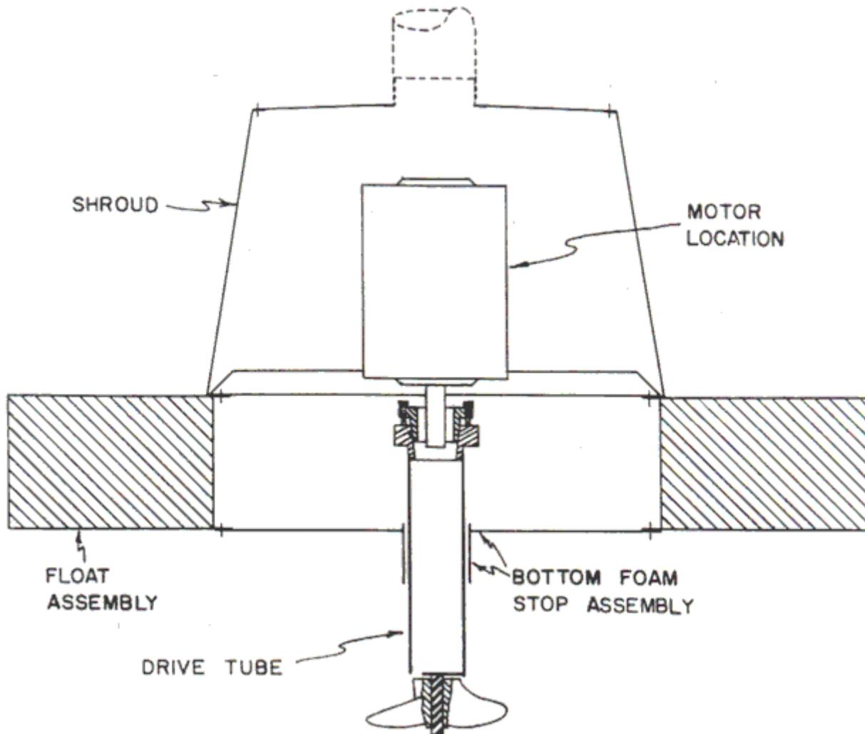
Similar aeration devices have been used for some time at a fixed position in underfloor oxidation ditches for swine confinement buildings. In this situation, where heat losses are small, stable liquid temperatures have been maintained in the thermophilic range of 110°F to 120°F. Such temperatures have been maintained throughout the winter without the addition of supplemental
